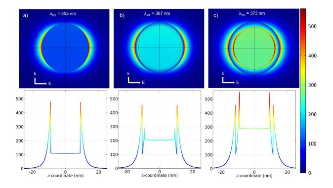
**Figure 5.** Electric field distribution maps  $(|E|/|E_0|)^2$  for a) bare silver nanoparticle, b) silver encapsulated by a polymer shell of thickness 1.4 nm, alike Ag\_L4 and c) silver encapsulated by a polymer shell of thickness 2.4 nm, alike Ag\_L8. The field enhancement along the Z-axis, i.e. in the direction of polarization, is plotted below the corresponding field maps.
