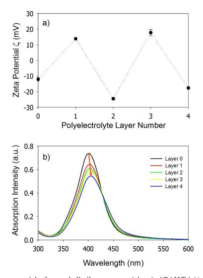
**Figure 1. a)** Zeta potential of core-shell silver nanoparticles Ag/(PAH/PAA)<sub>2</sub> as a function of adsorbed polyelectrolyte layer. **b**) UV-vis absorption spectra of core-shell silver nanoparticles as a function of adsorbed polyelectrolyte layer. The red arrow indicates the red shift in SPR peak position.
