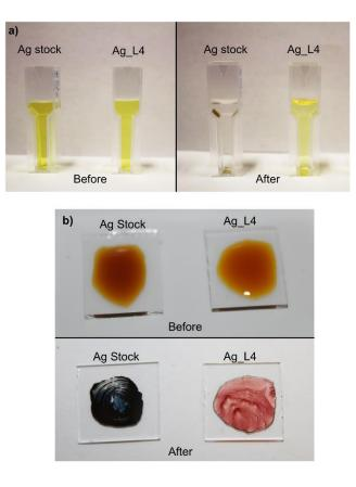
**Figure 4.** a) Photographic images showing the effect of salt addition on unprotected Ag *versus* protected Ag\_L4 colloidal nanoparticles and b) Photographic images showing the effect of hot air treatment on unprotected Ag *versus* protected Ag\_L4 nanoparticles.
