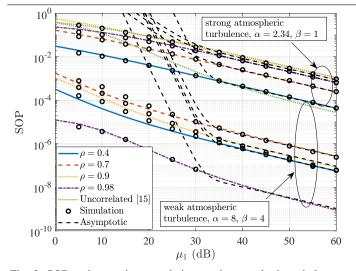
Fig. 2: SOP under varying correlations and atmospheric turbulences.
