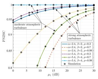
Fig. 5: PNZSC under varying correlation and channel conditions.
