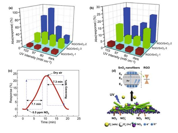
**Fig. 6** UV intensity-dependent response absolute value based on  $rGO/SnO_2$  sensors in **a** 3 ppm NO<sub>2</sub> and **b** 30 ppm SO<sub>2</sub>. **c** Enlarged part of response–recovery cureves of  $rGO/SnO_2$  sensor to 0.5 ppm NO<sub>2</sub>. **d** Sensing mechanism of  $rGO/SnO_2$  to NO<sub>2</sub> under UV illumination. Reproduced with permission [74]. Copyright 2019, Elsevier
