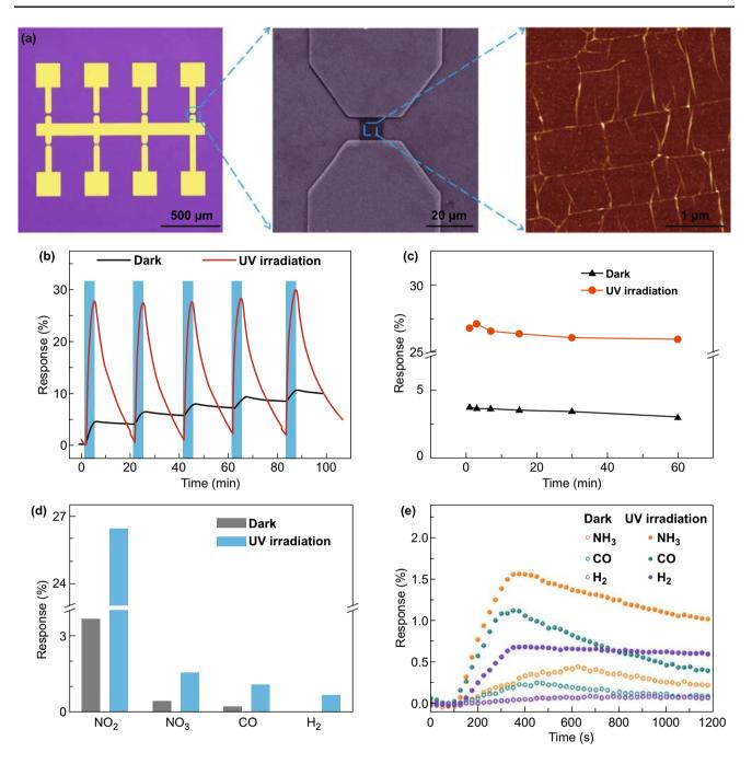
**Fig. 9** a Optical image of graphene sensors array, SEM image of graphene device, and AFM image of graphene. **b** Response and **c** stability test of graphene sensor to 100 ppm NO<sub>2</sub> in dark and UV illumination. **d** Selectivity bar diagram, and **e** transient response of graphene sensor to NH<sub>3</sub>, CO and H<sub>2</sub> at room temperature in dark and UV illumination. Reproduced with permission [87]. Copyright 2019, American Chemical Society
