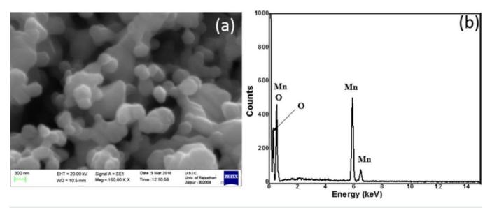
**FIG. 3.** LiMn<sub>2</sub>O<sub>4</sub> calcined at 800 °C for 14 h: (a) surface morphology and (b) EDX elemental spectra.
