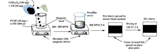
**FIG. 1.** Schematic of slurry preparation steps for spinel cathode LiMn<sub>2</sub>O<sub>4</sub>.
