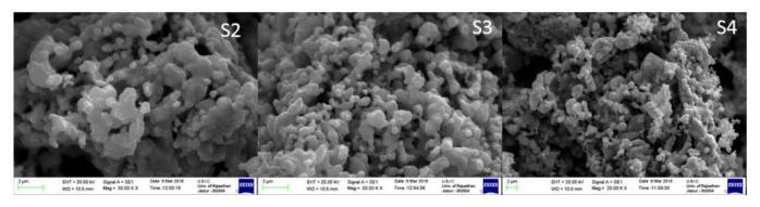
FIG. 5. SEM images of LiMn<sub>2</sub>O<sub>4</sub> slurry prepared with different stirring hours of (S2) 4 h, (S3) 5 h, and (S4) 6 h.
