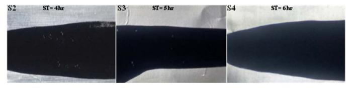
FIG. 4. Macroscopic view of the slurry prepared with different stirring hours (S2) 4 h, (S3) 5 h, and (S4) 6 h.
