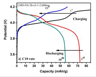
FIG. 7. Charge–discharge curve of slurry S3 for LiMn<sub>2</sub>O<sub>4</sub> at a current density of C/10.
