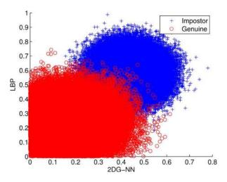
Fig. 7. Scatter plot shows that there is limited correlation between match scores obtained from LBP and 2DG-NN face recognition algorithms. Thus, score level fusion is expected to improve the matching performance.
