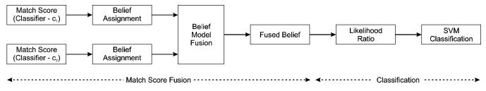
Fig. 1. Block diagram illustrating the steps involved in the proposed sequential match score fusion algorithm.
