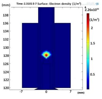
FIG. 6. Electron density at 4.5 kV/25 kHz (With flow).
