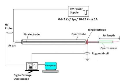
FIG. 2. Experimental set up of atmospheric pressure plasma jet using pin electrode configuration (with quartz sleeve).
