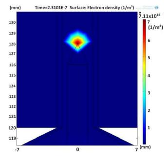
FIG. 5. Electron density at 4.5 kV/25 kHz (static condition).
