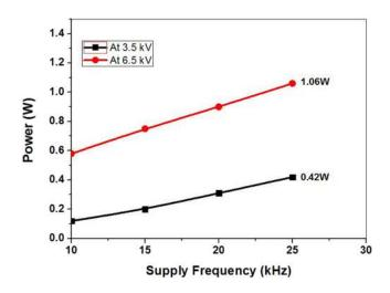
FIG. 17. Power consumed by the device Vs supply frequency at 3.5 & 6.5 kV.
