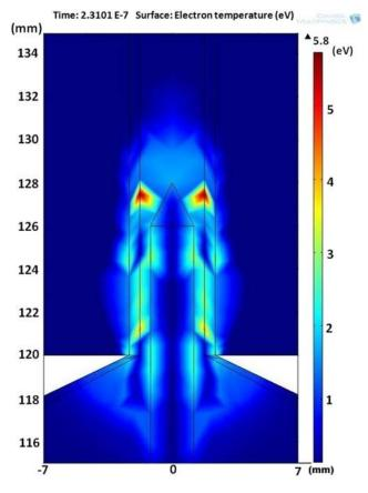
FIG. 8. Electron temperature at 4.5 kV/25 kHz (static condition).
