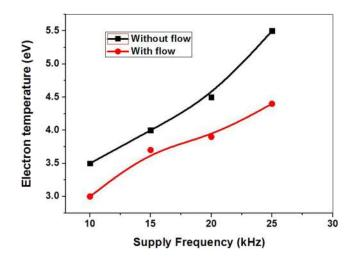
FIG. 10. Electron temperature Vs supply frequency at 4.5 kV.
