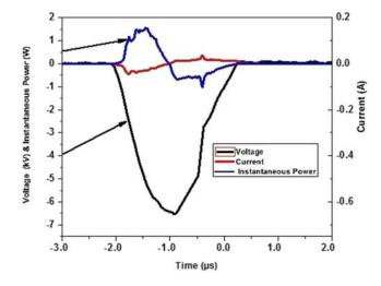
FIG. 18. Power consumed by the device 1.06W at 6.5kV/25kHz.
