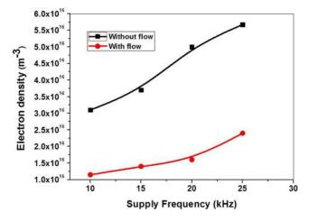
FIG. 7. Electron density Vs supply frequency at 4.5 kV.
