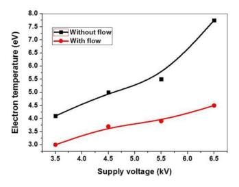
FIG. 12. Electron temperature Vs supply voltage at f = 25kHz.
