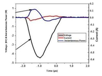
FIG. 16. Power consumed by the device at 4.5kV/25kHz.
