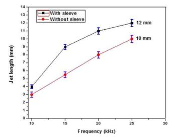
FIG. 20. Jet length Vs supply frequency at 4.5kV.
