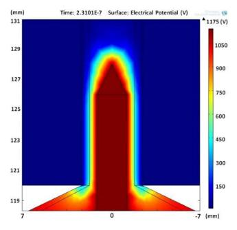
FIG. 14. Electrical potential reached at 4.5 kV/25 kHz (static condition).
