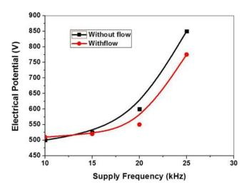
FIG. 15. Electrical potential Vs supply frequency at 4.5 kV.
