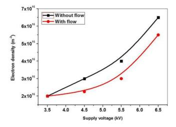
FIG. 11. Electron density Vs supply voltage at f=25 kHz.
