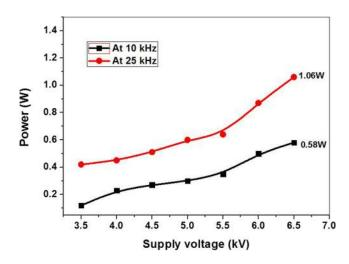
FIG. 19. Power consumed by the device Vs supply voltage at 10 kHz & 25 kHz.
