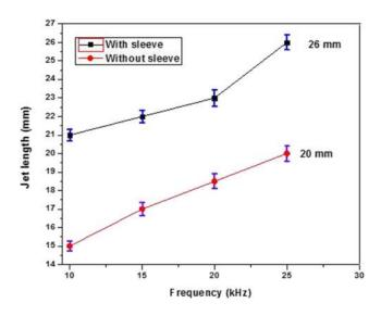
FIG. 21. Jet length Vs supply frequency at 6.5kV.
