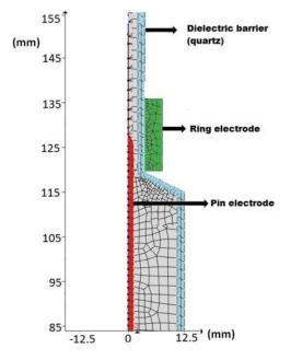
FIG. 4. Meshing of pin electrode APPJ using Finite element method (FEM).
