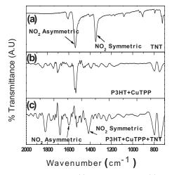
FIG. 4. FTIR spectra, wherein (a) is of pure TNT, (b) is for P3HT +CuTPP, and (c) is for P3HT+CuTPP after exposing to TNT vapors. Shifts in peaks are clearly seen in part (c) indicating the binding of the TNT molecules to the polymer composite.
