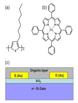
FIG. 1. (Color online) (a) Chemical structure of P3HT. (b) Chemical structure of CuTPP. (c) Structure of OFET.
