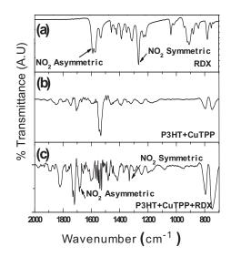
FIG. 3. Fourier transform infrared (FTIR) spectra, wherein (a) is of pure RDX, (b) is for P3HT+CuTPP, and (c) is for P3HT+CuTPP after exposing to RDX vapors. Shifts in peaks are clearly seen in part (c) indicating the binding of RDX molecules to the polymer composite.
