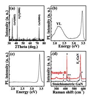
FIG. 1. (Color online) (a)  $2\theta - \omega$  HRXRD scanning curve of GaN film (sample-B) grown on c-sapphire. (b) Room temperature PL spectra of Ga deficient GaN film (sample-B). (c) PL spectra of typical stoichiometric GaN film and (d) Raman spectrum of GaN films.
