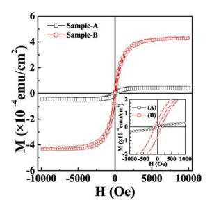
FIG. 3. (Color online) Magnetization versus magnetic field (*M*-*H*) at RT for GaN films with N:Ga  $\sim$  2.1:1 (sample-A) and 4.3:1 (sample-B). The inset presents the zoomed view of the *M*-*H* plot.
