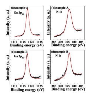
FIG. 2. (Color online) (a)-(b) XPS spectra of Ga  $2p_{3/2}$  and N 1s core level of sample-A and (c)-(d) XPS spectra of Ga  $2p_{3/2}$  and N 1s core level of sample-B.
