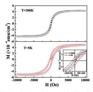
FIG. 4. (Color online) Magnetization versus magnetic field (*M*-*H*) for GaN film with N:Ga  $\sim$  4.3:1 (sample-B) at RT and 5 K. The inset shows the close up view of the *M*-*H* plot.
