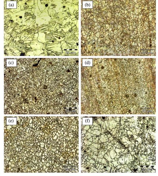
Fig. 1. Optical micrographs of the AZ31 Mg-alloy for (a) as-received plate and (b-f) caliber rolled at (b) 250 °C (c) 300 °C (d) 350 °C (e) 400 °C (f) 450 °C.
