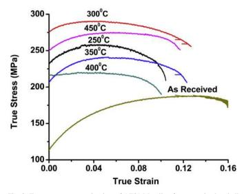
Fig. 2. True stress—true strain plots of AZ31 Mg-alloy for as-received and all the CR temperature conditions in plastic region.
