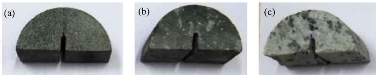
Fig. 3. Semi-circular bend specimens of (a) massive basalt, (b) giant plagioclase basalt, and (c) tonalite.
