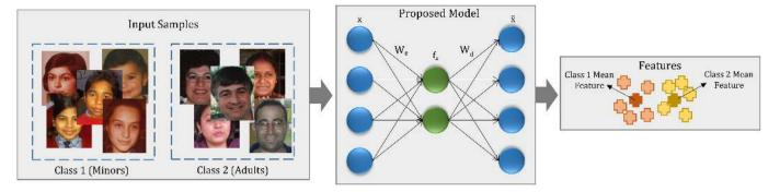
Fig. 5. Proposed Class Specific Mean Autoencoder. x and  $\tilde{x}$  represent the input and the reconstructed sample respectively,  $W_e$  and  $W_d$  denote the encoding and decoding weights, and  $f_x$  corresponds to the learned feature vector.
